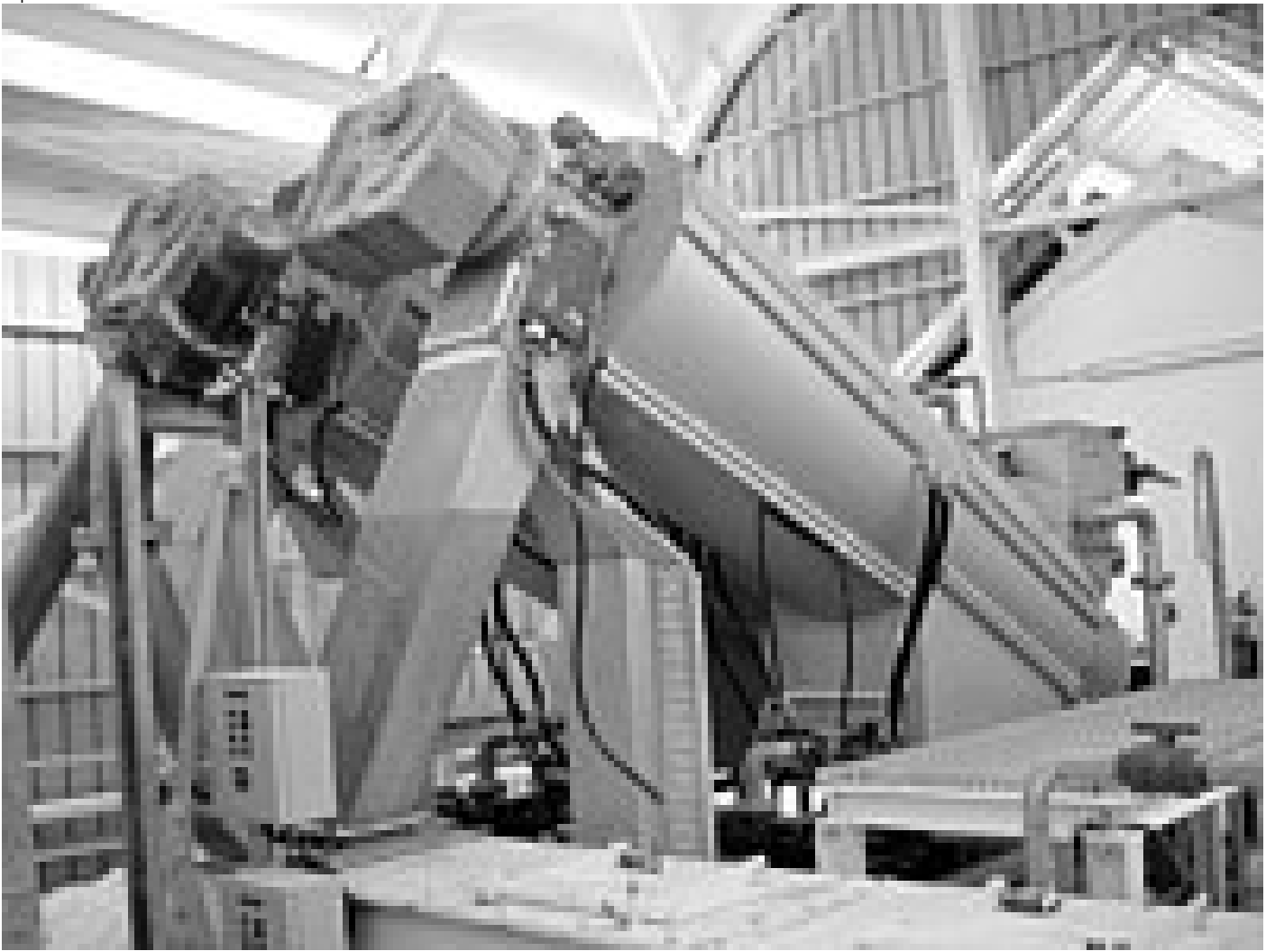
Sludge dewatering up to 40 % DS with HUBER ROTAMAT® RoS3
