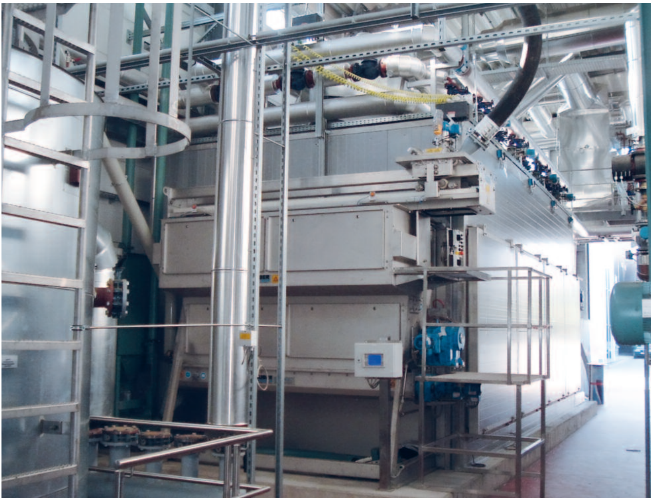
HUBER Belt Dryer BT: wet sludge feeding via pelletizer, dry material discharge via horizontal removal screw
